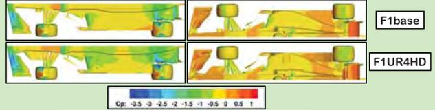
F1base vs F1UR4HD: Pressure Coefficient – top and bottom view
