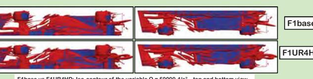
F1base vs F1UR4HD: Iso-contour of the variable Q = 50000 1/s<sup>2</sup> – top and bottom view
